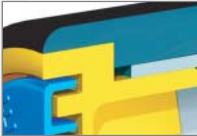
Ultra thick abrasion and corrosion resistant 12mm HDPE sleeve.
